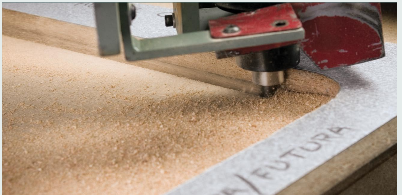
Precision sink cutout machines are used by fabrication shops.
